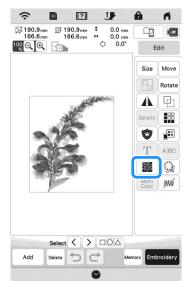
→ Stippling is automatically applied around the selected pattern.
