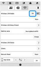
→ The machine begins to emit the wireless network signal.
