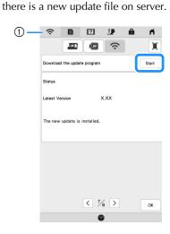
① When the wireless LAN key appears as , touching causes the machine to check if there is a new update file. If there is a new file, downloading begins.
